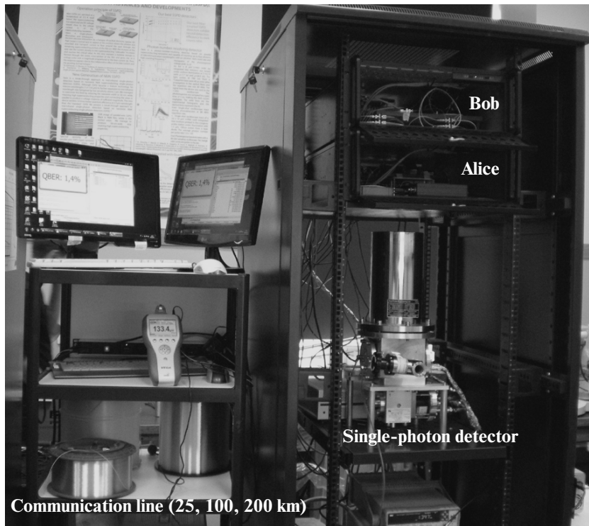
Fig. 3. Experimental setup of our subcarrier-wave quantum cryptography system. The figure shows the transmitting unit (Alice), the receiving unit (Bob), and the superconductor single-photon detector.
