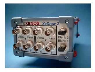
The XENOS *XeDraw 2* writer is a system that allows to design pattern data and to produce the respective deflection signals for beam steering of charged particle beams such as electron beams for semiconductor lithography applications or focused ion beam systems. Attached to a conventional scanning electron microscope, FIB, or dual beam tool, it upgrades the system to perform advanced nanolithography on semiconductor or other materials with this system.
