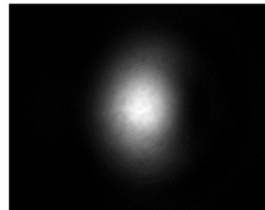
Infrared image of TEM00 laser output
