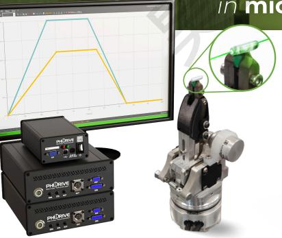
Phi Drive's wrist can be mounted on commercial robots to enhance **their precision and accurately** grab even the smallest samples.
