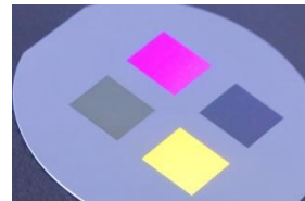
Silicon stamp with 4 pillar gratings. Pitch 200-400 nm, diameter 125-275 nm.
