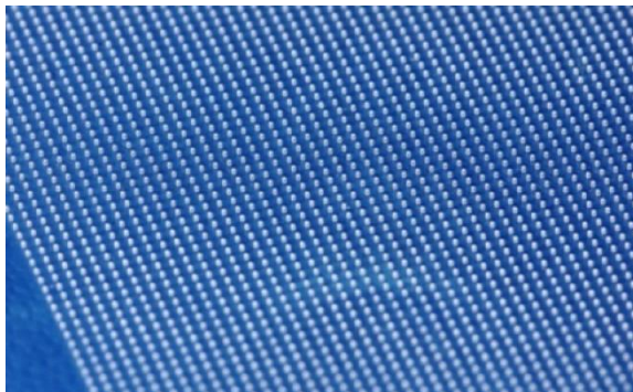
Pillar master stamp replicated in COP by CNI. 100 x 100 \mu\text{m} pillars.
