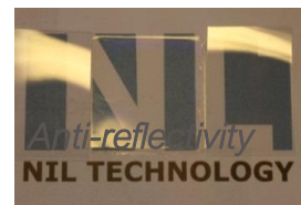
Image showing the functionality of the nanostructured polymer.
