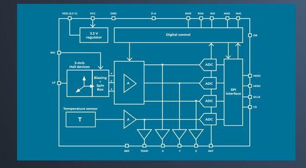
The MagVector<sup>™</sup> MV2 allows you to integrate a sophisticated magnetometer into your electronic system. A typical application is a sensor array for magnetic filed monitoring. The MV2 was developped by MPS Tech Switzerland Sàrl, in cooperation with Metrolab. Metrolab uses the same sensor in several of its products, and is now making this technology available to electronic systems designers.
