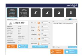
**PC control software -** For system integrators ML6600 is available as a subsystem which can be directly controlled with digital control signals through RS422, RS232 or Ethernet. Analog trigger signals are optionally available. ML6600 can also act as a stand-alone version, which comes with a PC software with elegant graphic UI.
