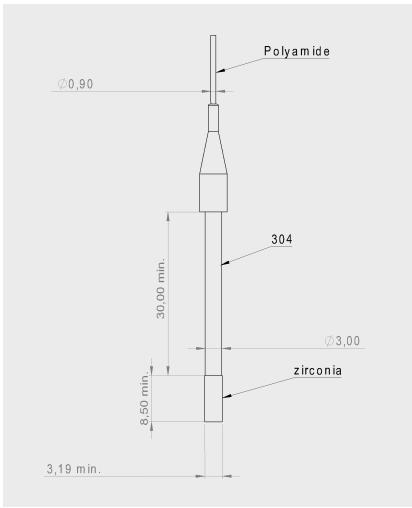
Figure 2 - Mechanical drawing
