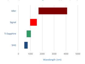
The Oria VIS includes four output ports which deliver 1) the OPO signal (990 - 1550 nm), 2) the SHG of the OPO signal (495 - 775 nm), 3) the OPO idler (1680 - 4000 nm), and 4) the depleted OPO signal (990 - 1550 nm). It incorporates a pump bypass which enables the selection of 100% of the OPO signal and idler (with no SHG of the signal) or 100% of the SHG of the signal (simultaneously with the undepleted OPO signal and 100% of the idler).
