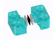
The Nanopore Flow Cell integrates the nanopore slot hosting a 5×5 mm squared and 200  $\mu$ m thick nanopore chip (black square in the exploded view . Two compartments for fluids (min 10  $\mu$ l, max 60  $\mu$ l volume) and the Ag/AgCl electrodes complete this mini flow cell with a size of only 18x28x10 mm.
