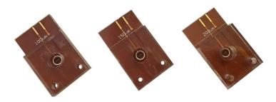
The BLMchips (top) are designed for biological pores. A layer of Polyimide, 12.5  $\mu$ m thick, hosts the micro hole available in two different sizes (100  $\mu$ m and 150  $\mu$ m). The BLMchip design allows an easy access to the buffer solution in both the chambers (60  $\mu$ l bottom, 60  $\mu$ l top) by pipetting. Ag/AgCl electrodes are integrated in the chip ready to be connected to eNPR device.
