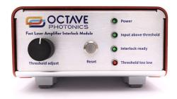
an optical amplifier system in the event of momentary or extended disruptions of the seed light. The FLAIM is a compact benchtop module that provides an adjustable input threshold for tripping the protection circuitry, shutting off the connected amplifier with a response time <1 ms. When used properly, the FLAIM can protect valuable nanophotonic components from accidental damage in laboratory environments.
