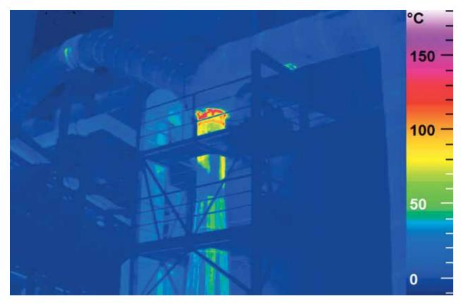
The sensitive thermal sensor technology detects faintest thermal abnormalities
