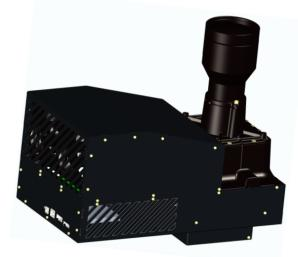
Chipset DLP670S | video pattern mode Display resolution 3840x2160 (XPR)1 Micromirror array size 2560x1600 Wavelengths (LED) 385 and 405nm Image resolution 4K Image size 195.84mm x 122.4 mm Standard lens native - 76.5 μm | 4K - 50 μm (other lenses available on demand) Optical output power (image) up to 6.5W Contrast ratio up to 1:175 ANSI Uniformity up to 95% acc. to IEC61947 (Lens-dependent)
