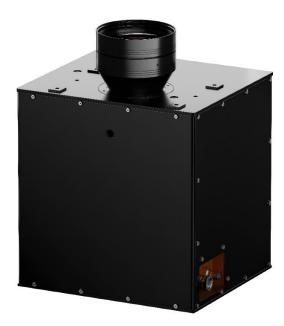
Chipset **DLP9000** Array resolution 2560x1600 Wavelengths (LED) 385, 405 and 460nm Standard lenses 2, 75, 84 and 162µm Optical output power up to 5W (wavelength-dependent) (image) Contrast ratio up to 1:400 ANSI up to 95% acc. to IEC61947 Uniformity (Lens-dependent)
