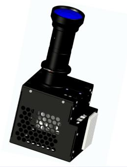
Chipset **DLP6500** Array resolution 1920x1080 Wavelengths (LED) 365, 385 and 405nm Standard lens 50, 84 and 100μm Optical output power up to 4W (wavelength-dependent) (image) Contrast ratio up to 1:300 ANSI Uniformity up to 95% acc. to IEC61947 (Lens-dependent)
