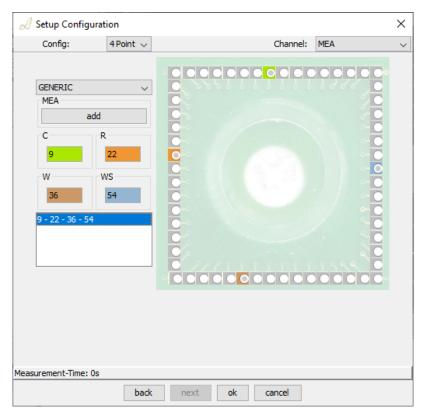
In the above example the measurement will be done with the channel configuration C9, R22, W36 and WS54.
