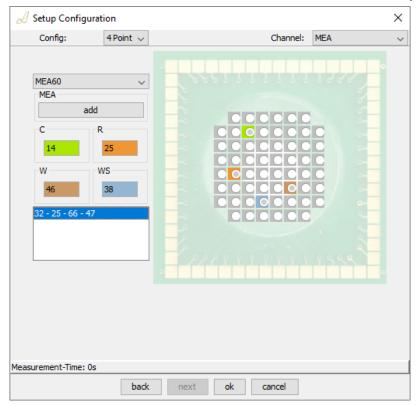
In the above example the measurement will be done with a MEA60 Chip and the channel configuration C14, R25, W46 and WS38.
