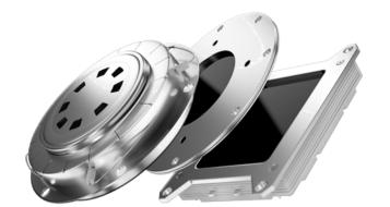
The singularity of Z-stack MCP produced by "Baspik" is that it has spaces between microchannel plates (having separate supplies) and it makes it possible to obtain the gain of more than  $1 \times 10^7$  (shevron) and  $1 \times 10^9$  (Z-stack) in contrast to other similar assemblies which do not have spaces between the plates and have the gain of  $1 \times 10^6$  and  $1 \times 10^8$  respectively.
