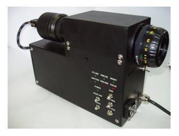
Camera is designed for fast process image registration in near infra-red and visible spectral ranges. Camera allows measurement of spatial-temporal parameters in streak and single-frame modes. Image from streak tube is recorded by CCD camera connected to PC. Software provides full control of camera functions and wide range of analyzing and processing tools for images.
