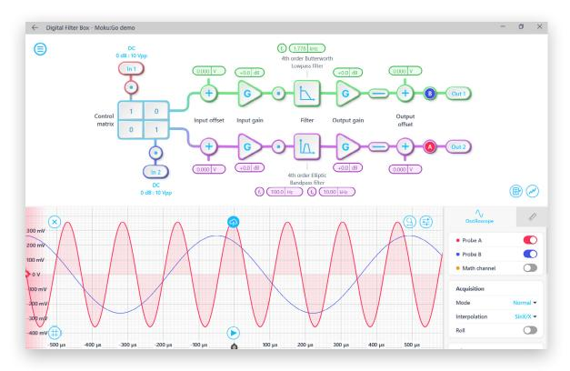
Sampling Rate 61.035 kHz, 488.28 kHz, or 3.9063 MHz
