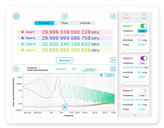
Frequency Range 1 kHz to 300 MHz Tracking Bandwidth
