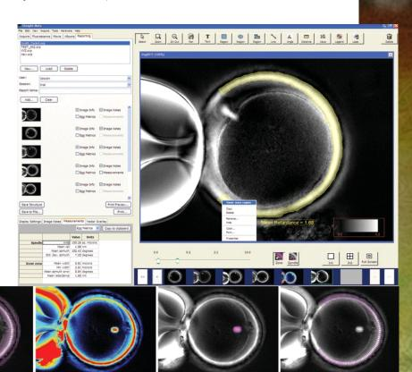
Oosight software visualization tools include (left to right): slow-axis orientation color map, orientation vector overlay, retardance color map, automated SpindleFinder $^{\text{\tiny{TM}}}$ , and automated ZonaFinder $^{\text{\tiny{TM}}}$ .
