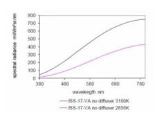
The ISS-17-VA can be operated at both color temperatures:2856K and 3100K
