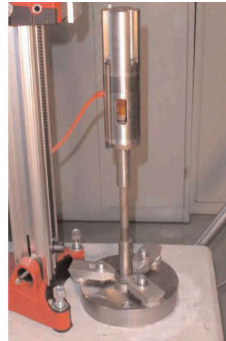
Figure 10: Test set up using a single output piezo-shock-generator with seismic mass for impulse reflection.
