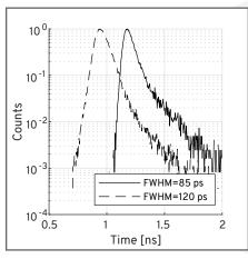
Excellent timing jitter with a FWHM of <120 ps for wavelengths between 510 and 785 nm.
