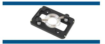
**IPZ Sample Holder Single Slide** 35 mm Petri Dish Accepts a standard 1 x 3 slide, or a 35 mm petri dish IPZ-4001
