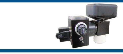
ASI's PhotoTrack solves the problem of tracking a moving specimen. Combined with ASI's closed loop DC servo motor XY stages, PhotoTrack allows you to keep your free-moving samples in your field of- view (FOV) no matter where they want to go. PhotoTrack uses a low-light-level rapid position sensing quadrant PMT sensor to monitor a bright reference spot on the target. It then commands the XY stage to maintain that spot in the center of a microscope's field-of-view.
