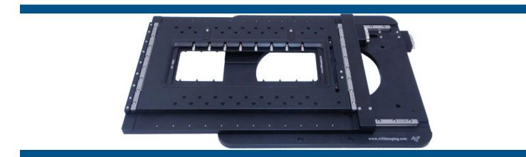
The MS-2500-Ti XY low-profile stage has been specifically designed to provide 100 mm (4") of Y-axis travel with an extended 250 mm (10") of X-axis travel. This extended travel makes for easy robotic loading or for holding more samples per stage insert. The MS-2500 stage accepts either standard 160×110 or wide 283×110 stage inserts. Total stage thickness is only 54.1 mm (2.13"), and only 29.3 mm (1.16") from its flat obstruction-free top to its bottom mounting surface.
