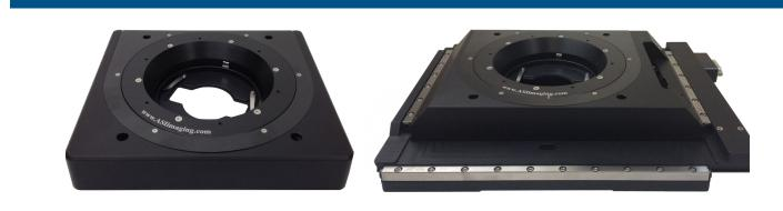
The PRS-1000 Precision Rotary Stage utilizes ASI's proven precise control through the use of closed-loop DC servomotors and angle encoded out drive. The low profile design with the ability to be integrated into our MS-2000 XY stages offers flexible usage. Standard versions have a ø 95 mm clear through aperture, use all of ASI's C size inserts, and have M3 tapped holes on 125 mm D.B.C. The PRS-1000 is also available with solid top plates for vacuum applications and M6 on 25mm centers.
