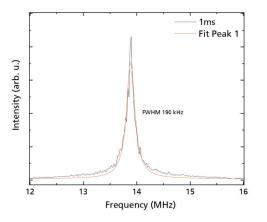
1 ms beatnote with Ti:Sapphire laser measured to have 110 kHz linewidth. Lorentzian fit has FWHM 190 kHz. REMOTE-Rb linewidth from this plot is 80 kHz @ 1 ms (locking to Fabry-Pérot interferometer, >200 finesse 1.5GHz FSR).
