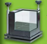
orthogonal axes. It is set in a housing that includes two adjustment knobs for leveling and aligning the Tool Cube.
