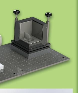
**Optical Testing.** PLX electronic autocollimators can be used for testing various optical components. Some can be measured directly, and others would require the use of supplemental optics.
