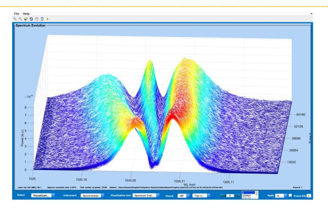
Spectral evolution of a supercontinuum laser during turn on event captured by COMET spectrometer.
