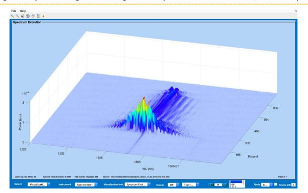
500 single-shot spectra during a Q-switching event is captured at 25 Million frames/sec over 20 μs.
