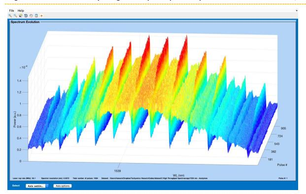
Single-shot transient of Acetylene gas absorption spectra captured at 36.1 Million frames/sec
