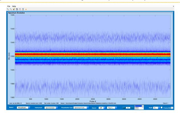
Spectral evolution of an unstable laser during a non-linear process analyzed by COMET software.
