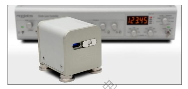
The MOGLabs LDL Littrow External Cavity Diode Laser is a research quality laser for advanced applications in atomic and quantum physics.
