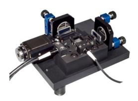
Interference is generally considered to be a wave phenomenon. Curiously it also works with single quantum objects. Use the quED-MI Michelson Interferometer add-on together with the quED to show that this is the case.
