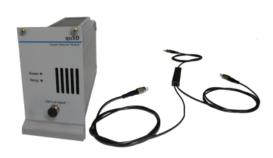
Explore the particle nature of single photons with the quED-HBT add-on for the quED. You can perform the "Grangier-experiment" with this Hanbury Brown & Twiss setup or build your own quantum random bit generator.
