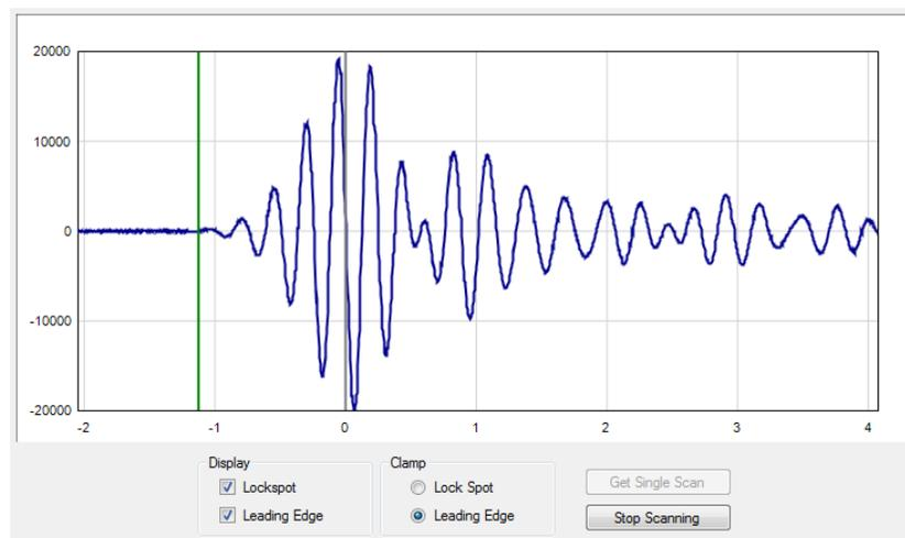
**Fig. 2-14: Waveform scan captured at 4 ps resolution**
