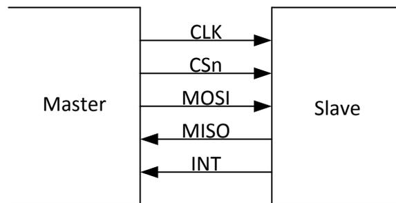
**Fig. 4-13: SPI interconnect signals**
