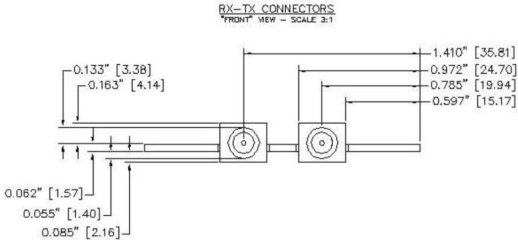
**Fig. 5-5: Locations and dimensions of RF SMA connectors**
