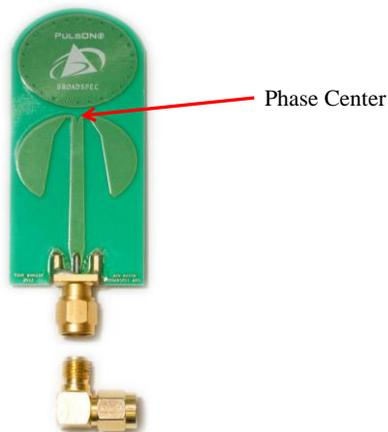
**Fig. 7-1: Broadspec antenna with phase center indicated**
