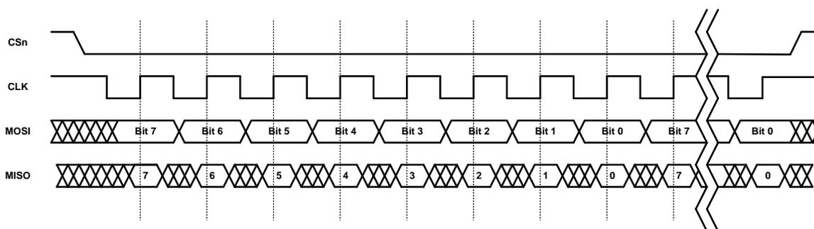
**Fig. 4-14: Signaling timing diagram**
