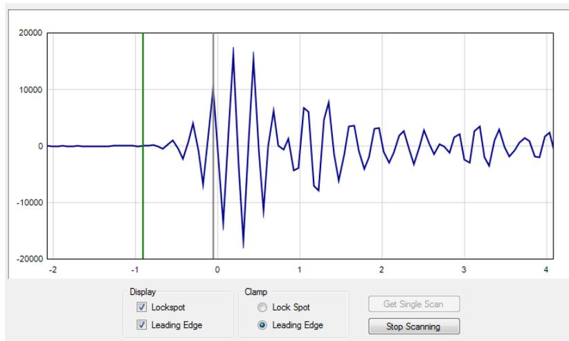
**Fig. 2-13: Waveform scan captured at 61 ps resolution**
