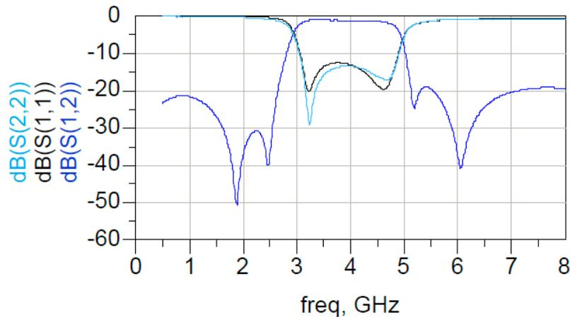
**Fig. 4-20: Characteristics of a single bandpass filter**
