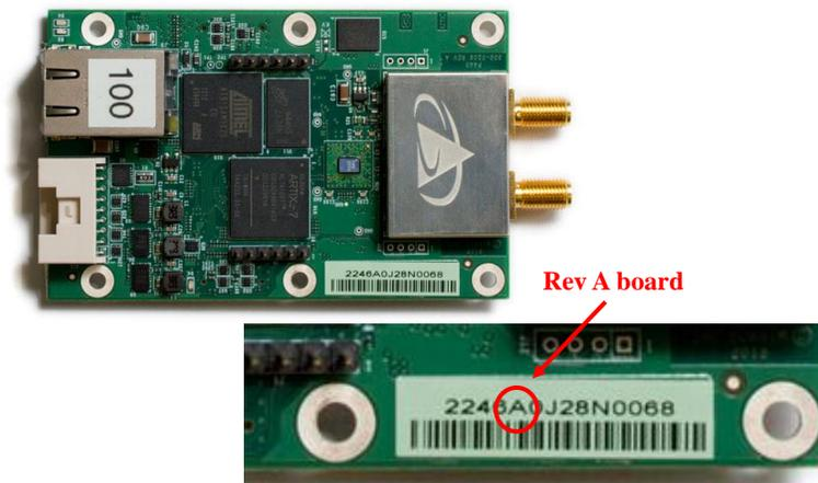
**Fig. 6-4: P440 Version indicated in bar code. Unit shown is a Rev A board.**
