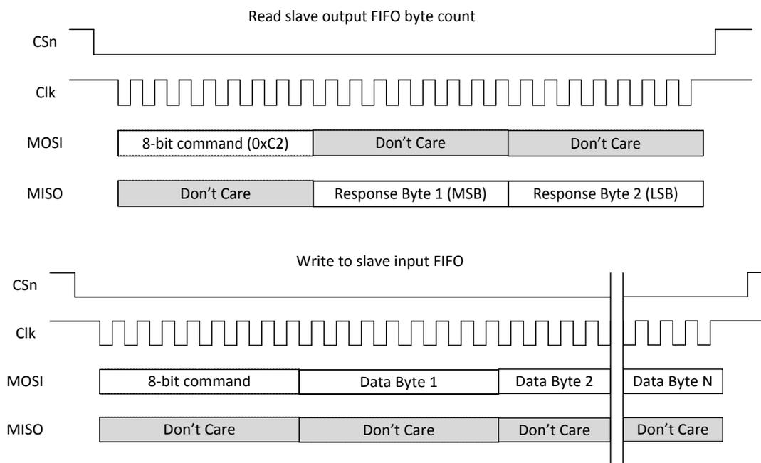
**Fig. 4-16: Timing diagrams**
