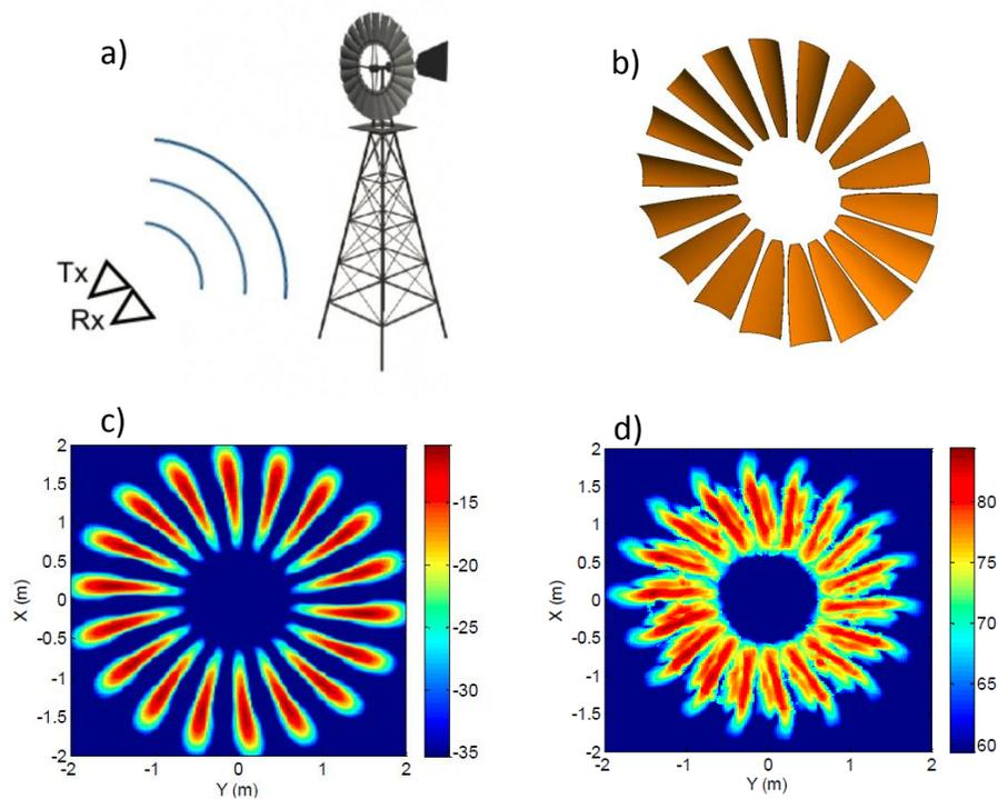
**Fig. 2-11: ISAR image of rotating windmill blades – (a) test setup (b) windmill blades (c) blades as modelled (d) blades as imaged by the ISAR**
