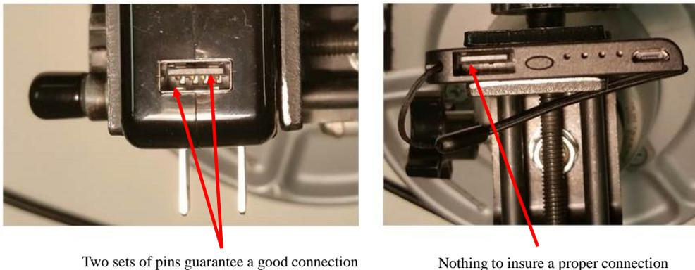
**Fig. 4-26: Superior connections (left) and inadequate product (right)**
