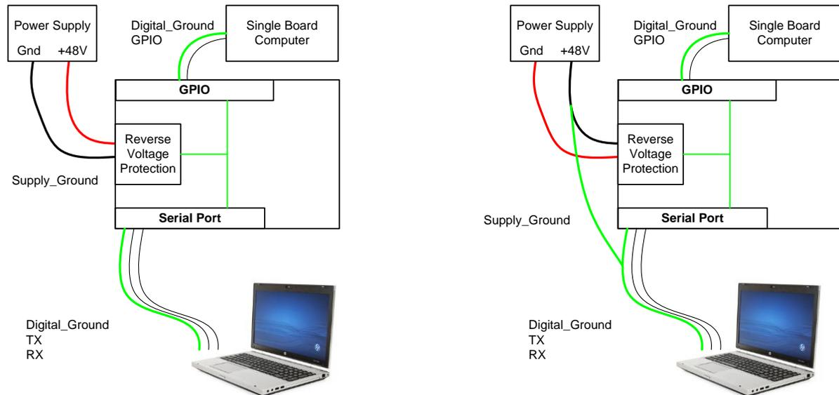
**Fig. 4-10: Properly connected configuration (left), dangerous configuration (right)**
