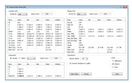
Fig. 2-8: Display of representative data computed and reported by the Location engine to RangeNet GUI
