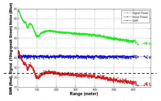
Fig. 6-1: Fresnel cancellation at 100 m can limit performance. If the SNR required to operate was 23 dB as shown by the black line, then the radio will work out to 210 m but not between 90 and 120 m.
