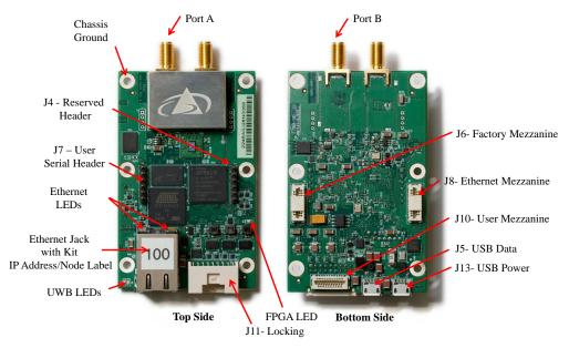
Fig. 4-1: Top and Bottom assembly drawing of the P440 highlighting key interfaces
