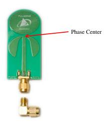
Fig. 7-1: Broadspec antenna with phase center indicated
