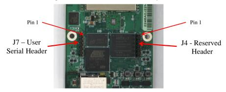
Fig. 4-9: User Serial pinouts
