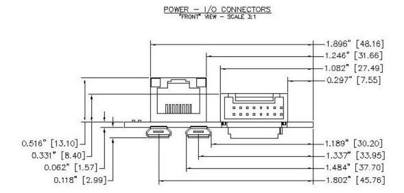
Fig. 5-4: Locations and dimensions of Power and I/O connectors at the rear of the P440
