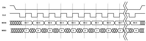
Fig. 4-14: Signaling timing diagram
