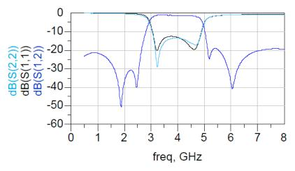
Fig. 4-20: Characteristics of a single bandpass filter
