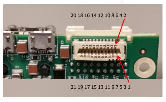
Fig. 4-8: J10 Mezzanine connector pinouts
