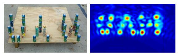
Fig. 2-10: SAR image of soda cans arranged to form the letters UAH
