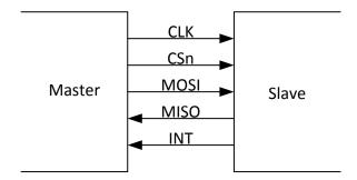
Fig. 4-13: SPI interconnect signals
