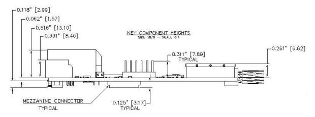
Fig. 5-3: Components which limit vertical height
