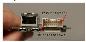
Fig. 4-7: J11 Locking connector pinouts
