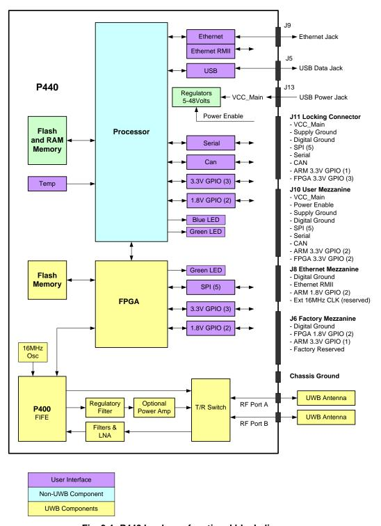
Fig. 3-1: P440 hardware functional block diagram
