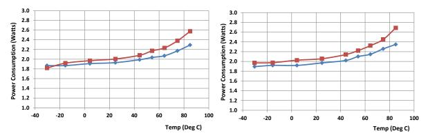
Fig. 4-11: Power Consumption as a function of board temperature for two representative P440s (red and blue) when operated as a transmitter (left) and as a receiver (right)
