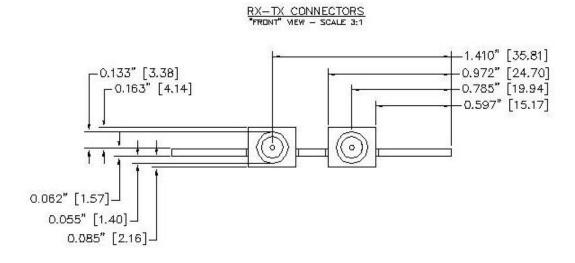
Fig. 5-5: Locations and dimensions of RF SMA connectors
