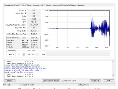
Fig. 2-3: Typical waveform as displayed by the GUI
