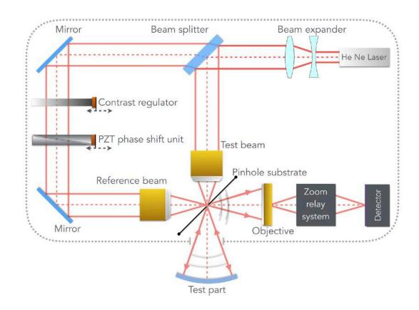
Two-beam phase shifting point diffraction interferometer provides a major advantage over other schemes by availing two independently steerable beams. Here, the test beam and reference beam are perpendicular to each other, where the intensity of the reference can be regulated. Concave shapes can be measured directly, whereas other kinds of optics are measured using a non-precise accessory.
