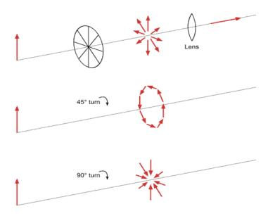
Radial polarization can be changed to azimuthal one by rotating segmented waveplate at 45 degrees. Direction of radial polarization becomes the opposite one by rotating the waveplate at 90 degrees.
