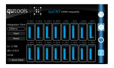
The definition of an entangled state in quantum physics can be rather simple: Two quantum objects cannot be described separately, only together. To show that a quantum system is entangled, the value of the Bell inequality (here, the CHSH equation) is determined by measuring the coincidence rate at 16 different polarizer settings. If the value is above 2, the state is entangled.
