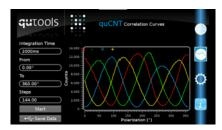
Polarization entangled states show correlations for all different combinations of the polarizer settings. You can fix one polarizer at 0° (horizontal, in the screenshot red), 45° (yellow), 90° (vertical, blue), 135° (green). The other polarizer is rotated. This shows the "non-classical" correlations of entangled photons.
