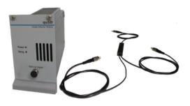
Explore the particle nature of single photons with the quED-HBT add-on for the quED. You can perform the "Grangier-experiment" with this Hanbury Brown & Twiss setup or build your own quantum random bit generator.
