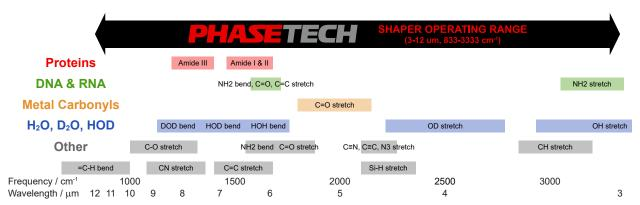
The QuickShape operates at wavelengths covering the most-studied vibrations of proteins, DNA & RNA, metal carbonyls and water. Extended wavelength ranges are also available by request.
