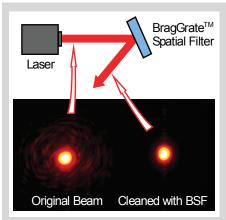
Spacial filtering of 632.8 nm HeNe laser with BSF
