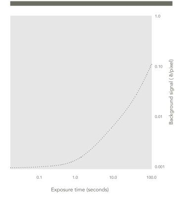
Figure 1 Mean signal of HNü 512 dark frames as a function of exposure time Data measured at 10MHz with an EM gain of 1000 at -85 °C
