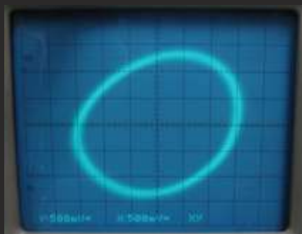
a) IQ (quadrature) mixer output (while unlocked)
