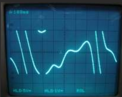
b) Phase memory analog output (while unlocked). The amplitude of 10Vpp corresponds to full 8192 cycles!
