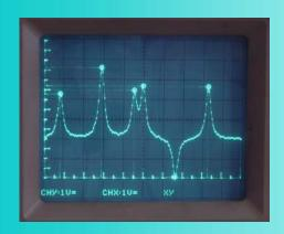
Doppler-free absorption saturation spectrum of the Cs-D<sub>2</sub> line
