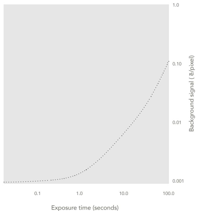
Figure 1 Mean signal of HNü 512 dark frames as a function of exposure time
