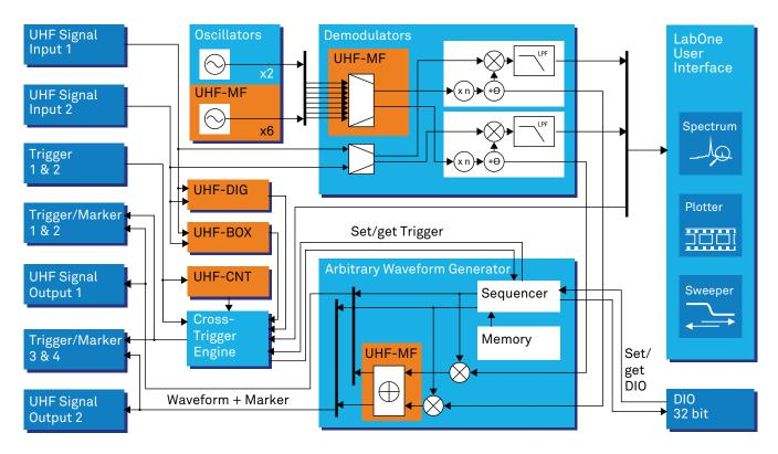
Orange color in the diagram indicates optional upgrades. The UHF-AWG Arbitrary Waveform Generator is available both as a stand-alone instrument and as an upgrade option to the UHFLI Lock-in amplifier.
