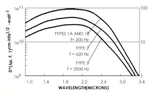
Typical Spectral Response Shows How Devices Can Be Tailored to User Spectral Requirements.
