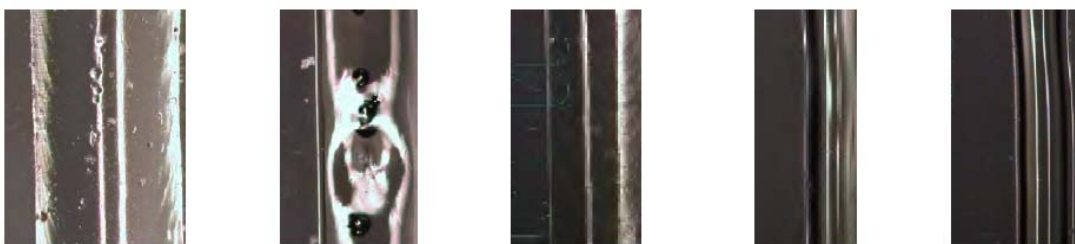
Figure. 6 Optical microscope images of the lines of melted PMMA material made on surface of the sample with different scanning speeds. The laser power – 3.45 W.
