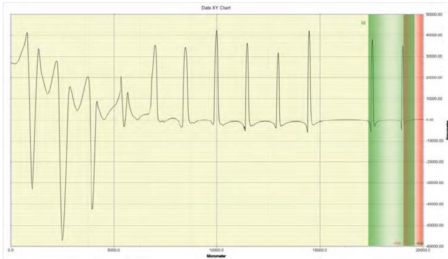
Figure. 7 The crosscut height measurements with DEKTAK 150+ stylus profiler. Scan speed from left to right: 1, 2, 3, 4, 5, 6, 7, 8, 9, 10 mm/s. Laser power – 3.45 W;
