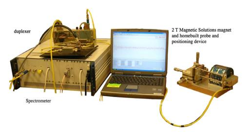
Fig. 1. Picture of our table-top laser-lathe lithographically microcoil NMR setup, which consists of a Tecmag spectrometer for control, a small Halbach magnet, and an RF probe with a 360 µm microcoils.
