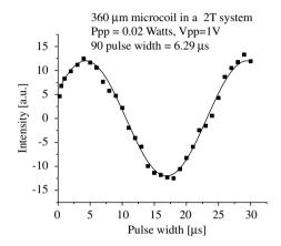
Fig. 5. Nutation curve of the portable RF probe with 360  $\mu m$  OD microcoil for 0.02 W of power.
