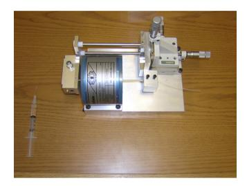
Fig. 2. A picture of the Halbach magnet and RF probe with a  $360 \,\mu\text{m}$  microcoil on a translation stage, which is used to map out the magnetic field of the Halbach magnet.
