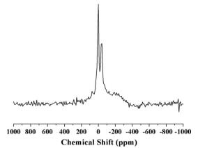
Fig. 6. <sup>19</sup>F spectrum in the optimal sweet spot of the magnet. The resolution is 17 ppm.
