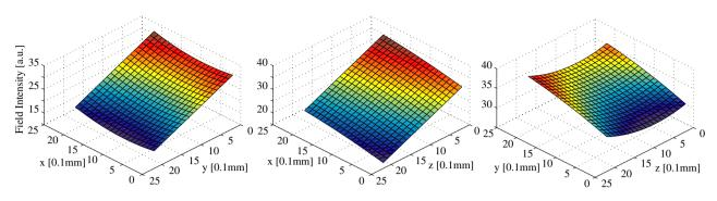
Fig. 3. 2D surface plots of the static field in the Halbach magnet.
