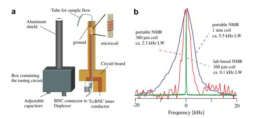
Fig. 4. (a) A Schematic of our first generation microcoil probe made on a circuit board. (b) NMR spectra taken from a homebuilt probe with a 360 µm RF microcoil for our 500 MHz system, a homebuilt probe made from a circuit board with a 1 mm and 360 µm RF microcoil for our portable 2 T Halbach magnet.
