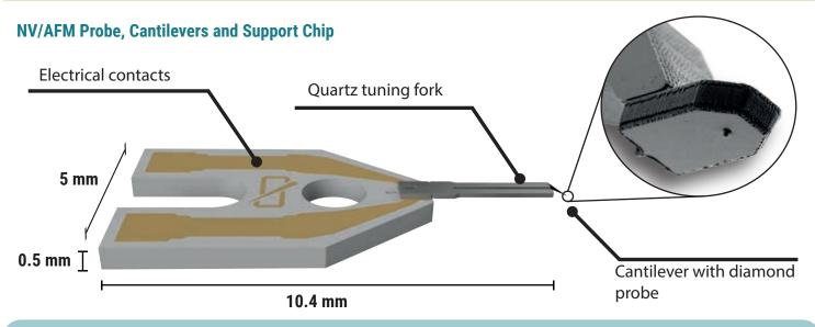
The Quantum Sensor Tips contain a high-quality diamond tip with a single embedded NV center mounted on a robust ceramic carrier plate. An integrated force-feedback sensor based on a quartz tuning fork provides safe distance control. Our quality control team ensures that only the top performing probes are selected for our customers.
