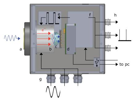
When the TRiCAM is mounted to a microscope or lens, the incoming light (a) is focused onto the entrance window of the image intensifier (b). The image intensifier converts the optical image to electrons, amplifies this electron image, and re-converts the electrons into photons. A fiber-optic taper (c) guides the amplified optical image to the CMOS module for registration and read-out (d).
