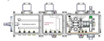
BaySpec mass spectrometers also benefit from a completely custom vacuum design that includes pump fabrication, chamber housings, and conductance limiters. These technologies allow our mass spectrometers to perform atmospheric sampling without sacrificing size or performance.
